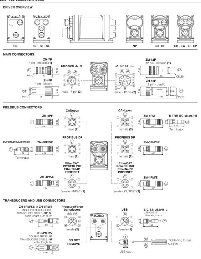
(1) Use of metallic connectors is strongly recommended in order to fulfill EMC requirements (2)
