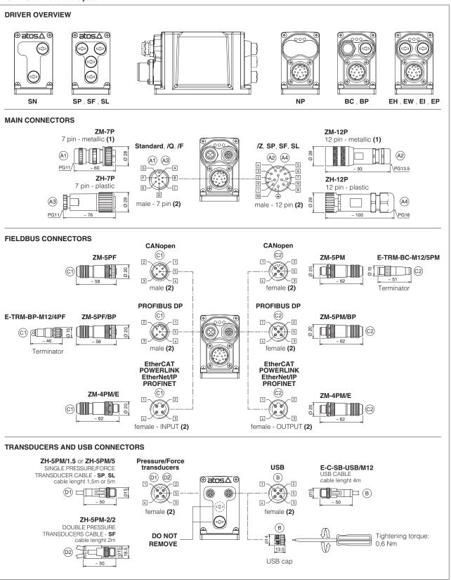
(1) Use of metallic connectors is strongly recommended in order to fulfill EMC requirements (2) Pin
