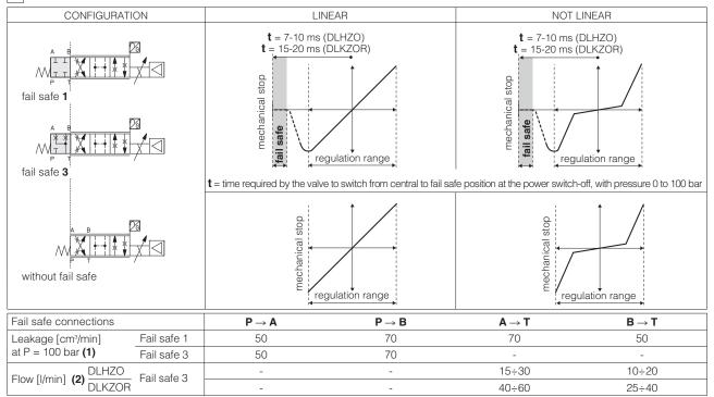
(1) Referred to spool in fail safe position and 50°C oil temperature
