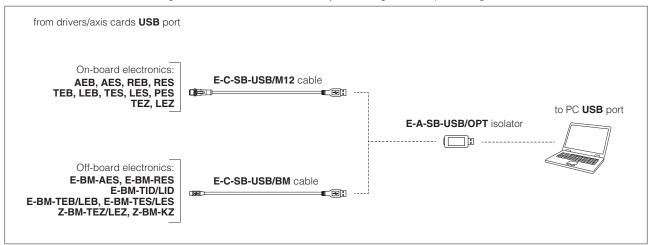
**WARNING:** drivers/axis cards USB port is not isolated! Use of USB isolator adapter is highly recommended for PC protection: wrong earthing connections may cause high potential difference between GNDs, generating high currents that could damage the PC connected to drivers/axis cards.
