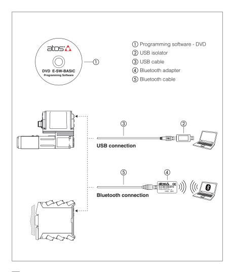
The E-SW and Z-SW programming software are supplied in DVD format and can be easily installed on a desktop or a notebook computer. The intuitive graphic interface allows:
